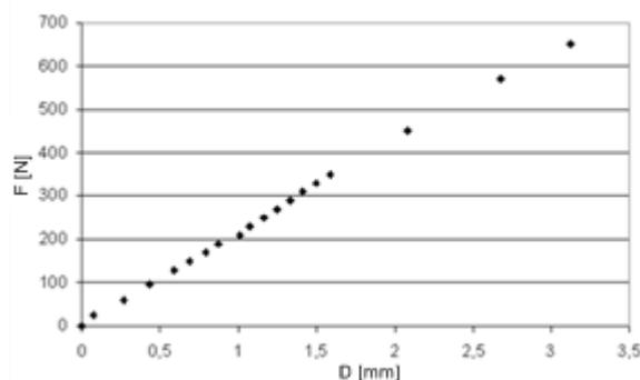
Fig. 8. Working platform dislocation chart for a system load towards the passive arm (measured perpendicularly to the force)
