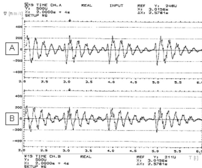
Fig. 9. Changes in platform speed in response to the driven force of 100N recorded by sensors A and B placed on the working platform
