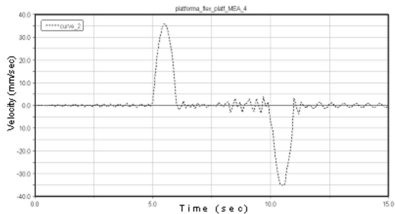
Fig. 16. Changes in speed (in the direction of the Z-axis), set for working platform during movement along a given trajectory at the speed of 0,02m/s (with changed values of rigidity of passive elements)
