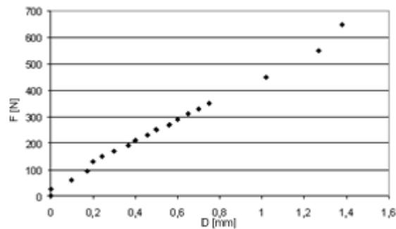
Fig. 7. Working platform dislocation chart for a system load towards the passive arm (measured in the direction of the force)
