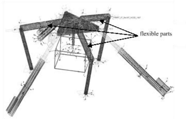
Fig. 15. Computational model of the machine drive system with flexible parts (elements of passive arms with increased rigidity)
