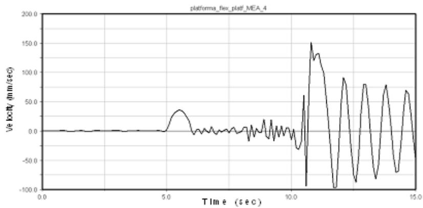
Fig. 13. Courses of changes in forces and speeds in the system (in the direction of the Z-axis) during working platform movement along a given trajectory with the speed of 0,02m/s
