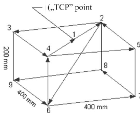
Fig. 11. Preset movement trajectory of a hypothetical tool („TCP” point)
