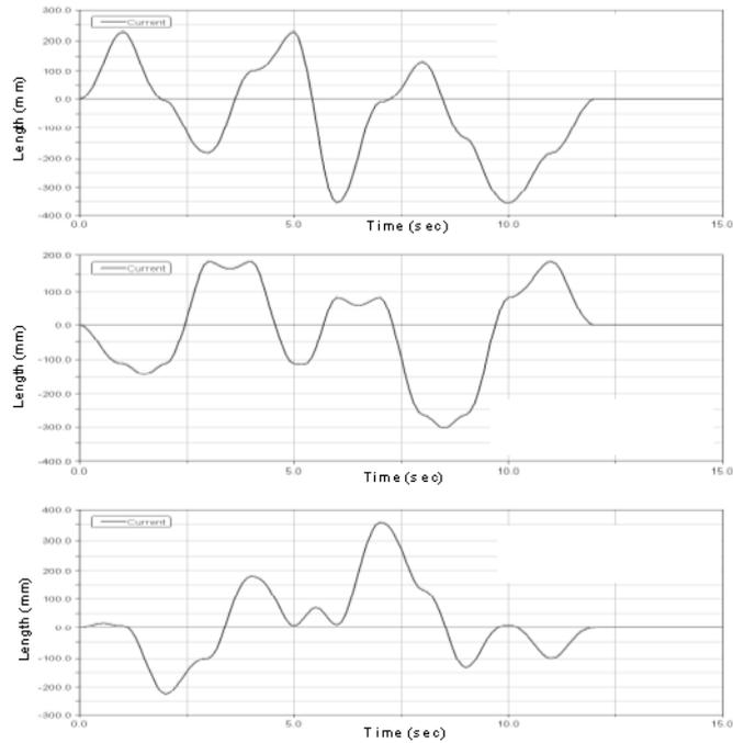
Fig. 12. Courses of feed movement components for with drawable kinematic couples
