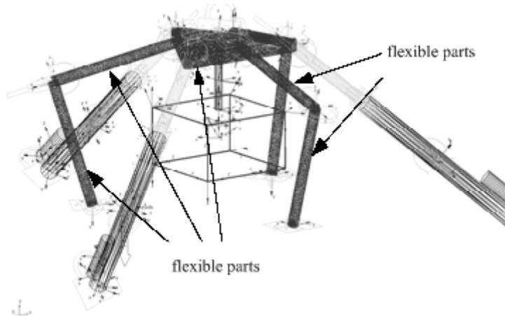
Fig. 10. A computational MBS model of a machine drive system with marked flexible parts
