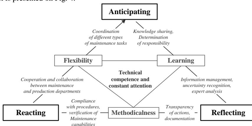
Fig. 4. The maintenance core task model [19]
