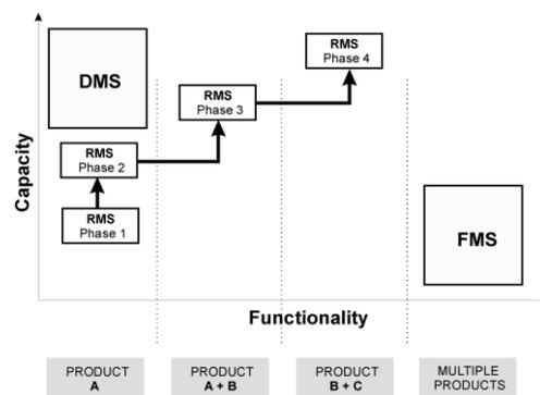
Fig. 5. Capacity and functionality of different forms of manufacturing systems [14]
