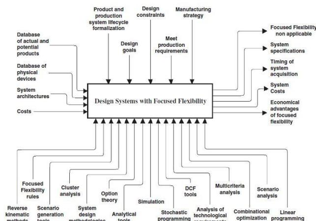
Fig. 6. Focused Flexibility Manufacturing Systems design diagram [16]
