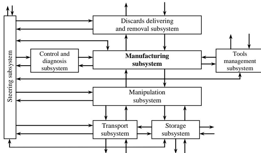
Fig. 3. A functional structure of an FMS [11]
