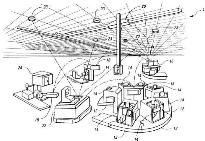
Fig. 4. An example of structure of Reconfigurable Manufacturing System [13]
